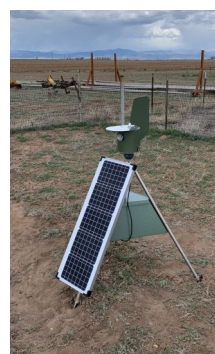
Figure 2: Burkard multi-vial cyclone sampler was set up in mid-May at the San Luis Valley Research Center to monitor potato foliar pathogen spore dispersal patterns.
